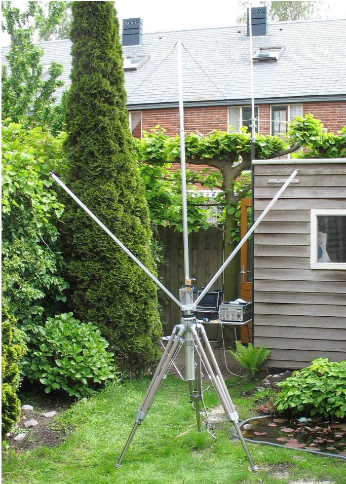
Photo 3.1. Noise measurement setup with magnetic loop antenna, datalogger and measurement receiver.
