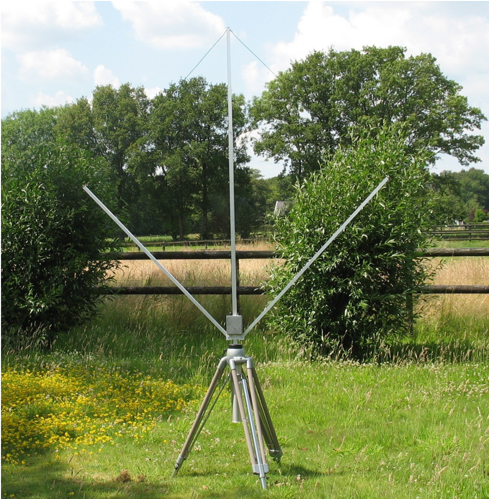
Photo 2.1. The low-band antenna unfolded. The vertical limb is retractable. The lower parts of the loop exists of square aluminium profiles wherein an aluminium rod is mounted as an inner conductor with screws on both ends. The upper parts are made of 1.5 mm diameter copper wire, isolated. In the lower corner the box with tuning and amplifier is situated.
