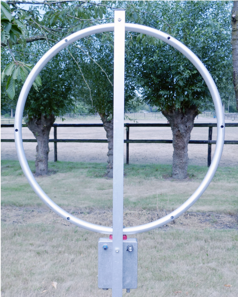
Photo 2.4. The high-band loop antenna. The basis is formed by a wheel-chair handle and is cut on the lowest part, and connected to the active part. Here the fine tuning potmeter and the band switch are mounted on the backside.
